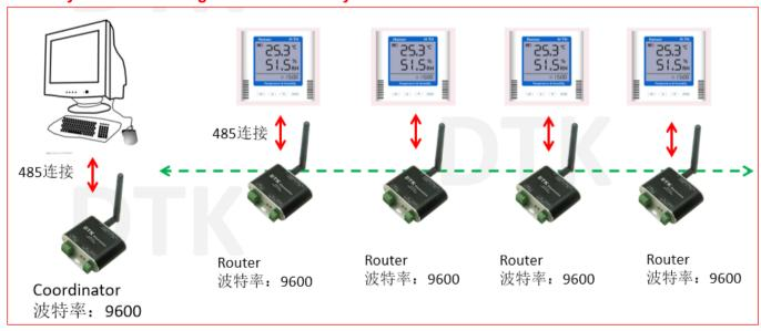
When configuring the Zigbee module, you only need to configure the coordinator. The Router module can automatically find the coordinator to join the network by pressing the function button 3 times, and obtain the preset parameters in the coordinator.
