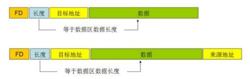
If the target address is FF FF, the broadcast is sent to all nodes.
