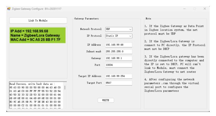
Run the "virtual serial port" software on the computer and virtualize this network port into a serial port, then you can operate this network port in the same way as a serial port, including setting some parameters of Zigbee
