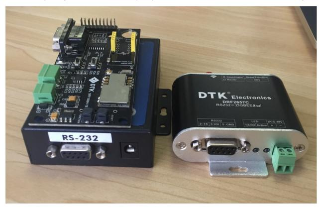
At this time, the module and the device should be cross-connected ( 2-3 , 3-2 , 5-5 ) Its essence is still TX-RX , RX-TX , GND-GND
