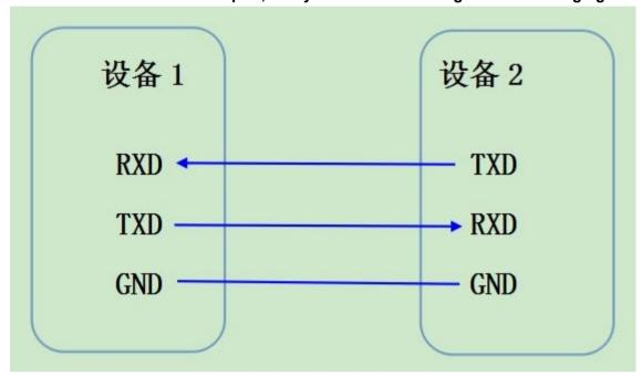
According to the above definition, there is a direct connection between the computer (or USB to RS232) and the module (DRF2657C):
