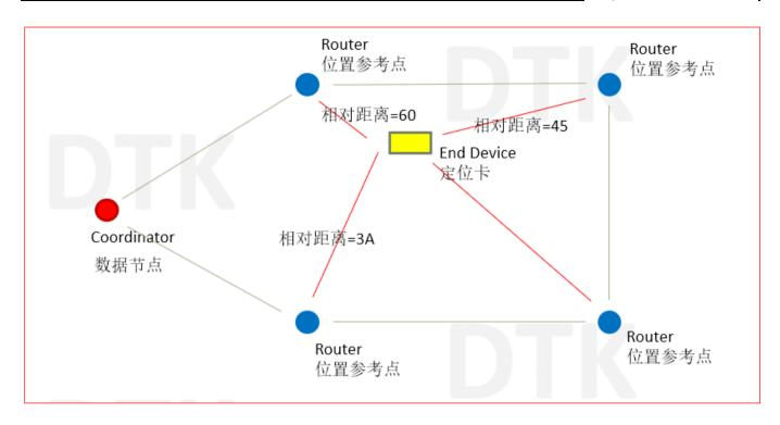
the positioning card (End Device) generates positioning data, it will send the positioning data to the nearest position reference point (Router), and the Router will automatically route the positioning data to the coordinator, and then the upper computer software will display the position of the positioning card. The positioning data format is as follows:
