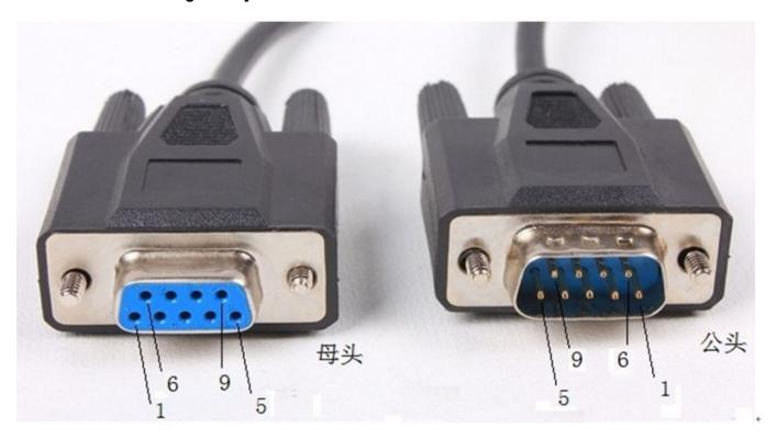
RS232 interface on the computer, or the USB to RS232 interface, is generally a male head:
