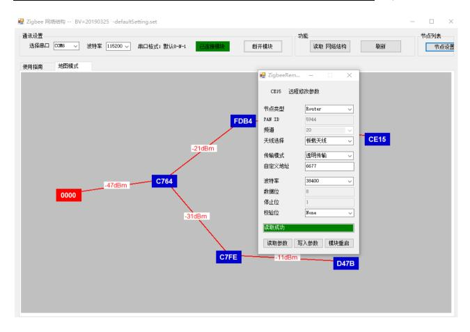
For example: modify the node type of CE15 node to: End Device
