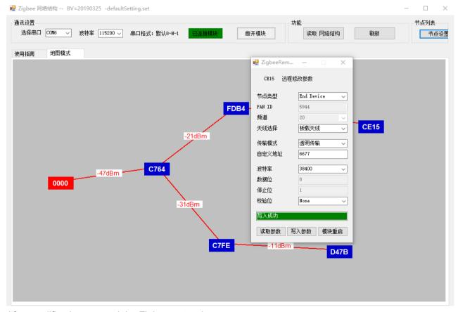
After modification, re-read the Zigbee network:
