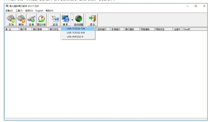
8. Automatically search out DRF2670C , click "connect virtual serial port", fill in the parameters, and "confirm";
