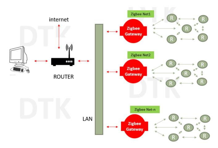
When the Zigbee gateway is connected to the computer through a router, the general configuration is:
