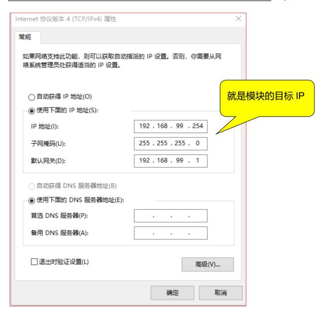
6. The IP address of the gateway ( DRF2670C ) and the computer is the target IP of each other. If it is not clear, please read out the corresponding parameters and fill in the form below:
