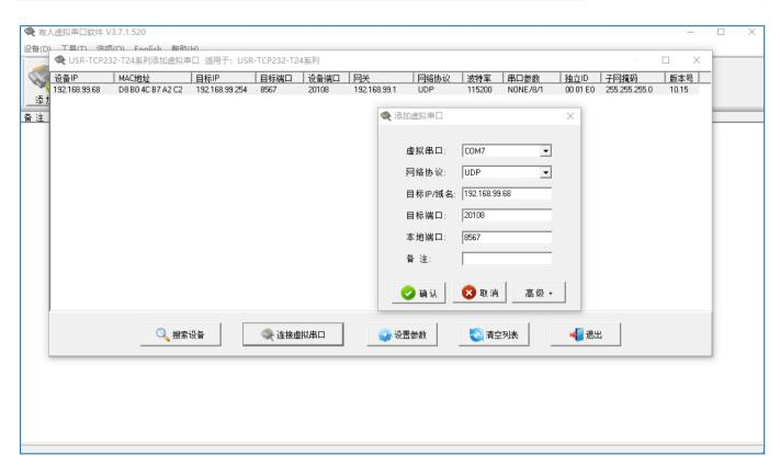
9, the virtual serial port is successfully created, check "Synchronous Baud Rate";
